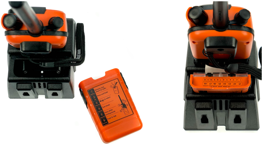
Figure 5 Radio in the charging bay and GMDS battery in the storage bay
